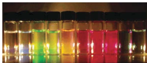
Fig. 5 Fluorescent core-shell silica nanoparticles incorporating organic dyes with different spectral characteristics, covering the entire UV-vis absorption and emission wavelengths. (Reproduced from ref. 31, with permission. Copyright 2005 American Chemical Society.)
